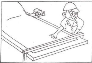
C) Push START button and the cutter will automatically cut the cloth that was laid across the track. If automatic lifters are included, the track will move up and down. If not, manually lift the track and allow the cloth to fall underneath before lowering track back to table.
